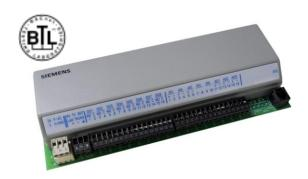
The Siemens BACnet PTEC Fan Coil Controller provides high performance Direct Digital Control (DDC) of pressure-dependent boxes, fan coil units, and induction units. The Siemens BACnet PTEC Fan Coil Controller can operate stand-alone or can be networked to perform complex HVAC control, monitoring and energy management functions and is designed to reside on any BACnet control system.
